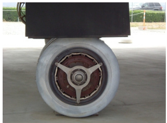
Main gear wheels were impregnated with aluminium powder to help protect them against heat at high speed.
