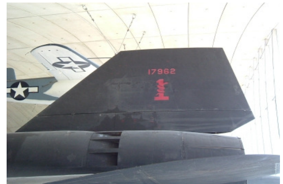
All moving Rudders canted inwards at 15 degrees. Note the tertiary doors - these closed above Mach 1.5.
