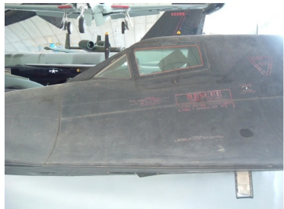
The front windshield knife edge device was installed to help dissipate heat generated from high speed flight.
