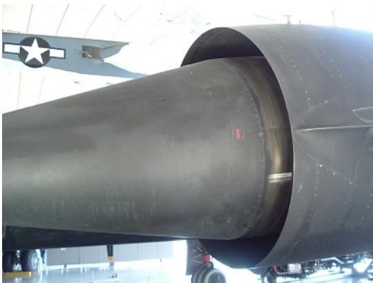
The intake spike and various other inlet devices. The intake shifted 26 inches and at Mach 3+ speeds accounted for 80% of engine thrust.
