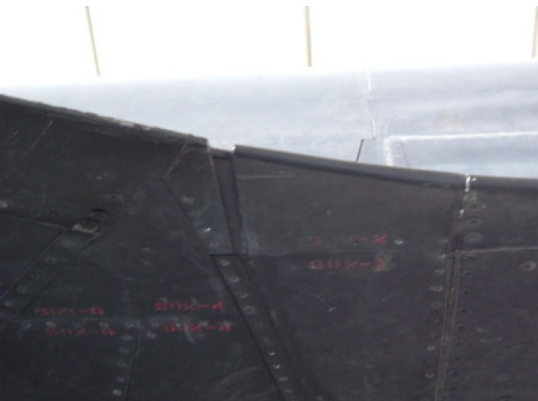
Wing heat expansion joint built in to the airframe.
